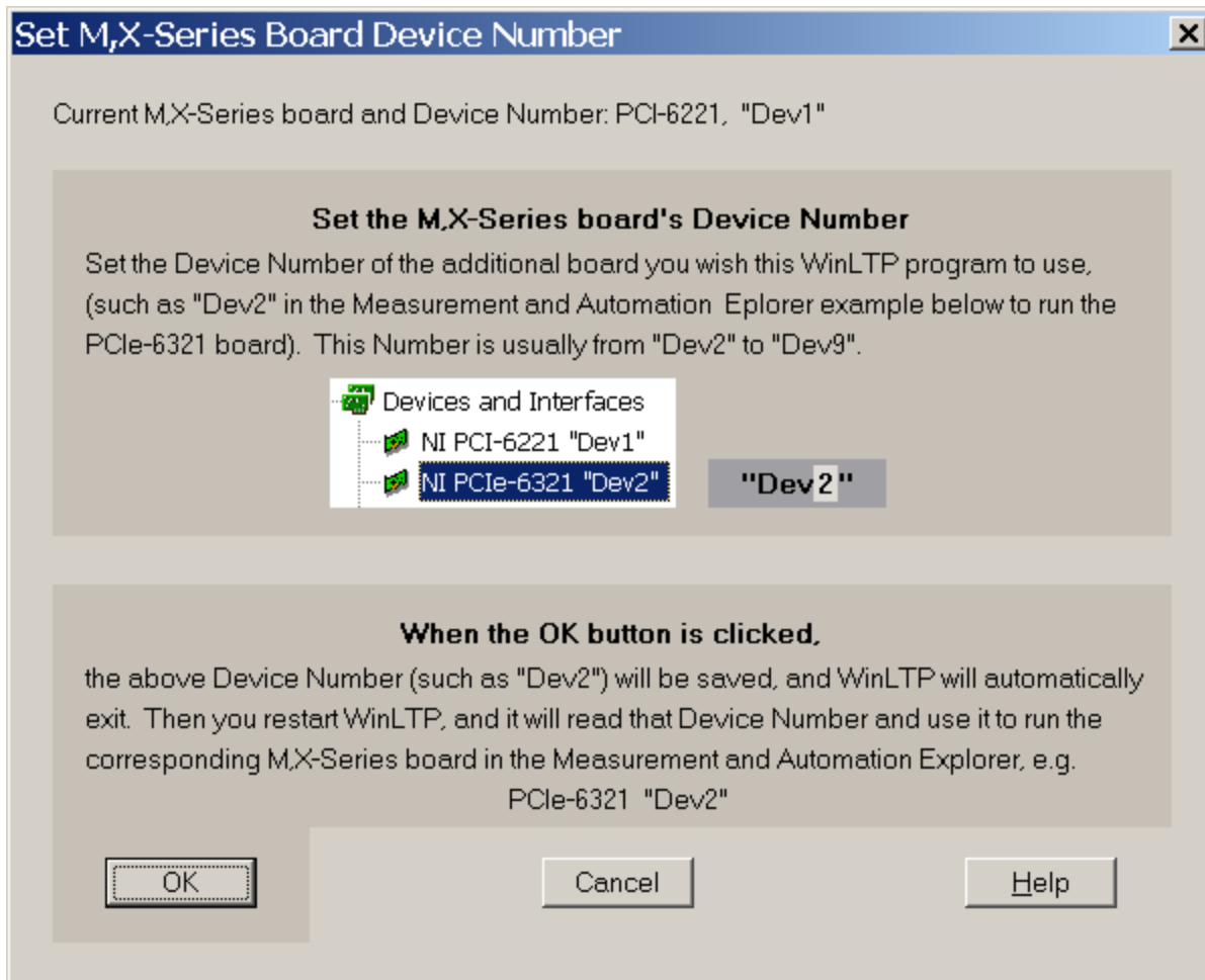
Fig 2.4.7.1. The Set M,X-Series Board Device Number dialog box used to set the Device Number of an additional M- or X-Series board.
