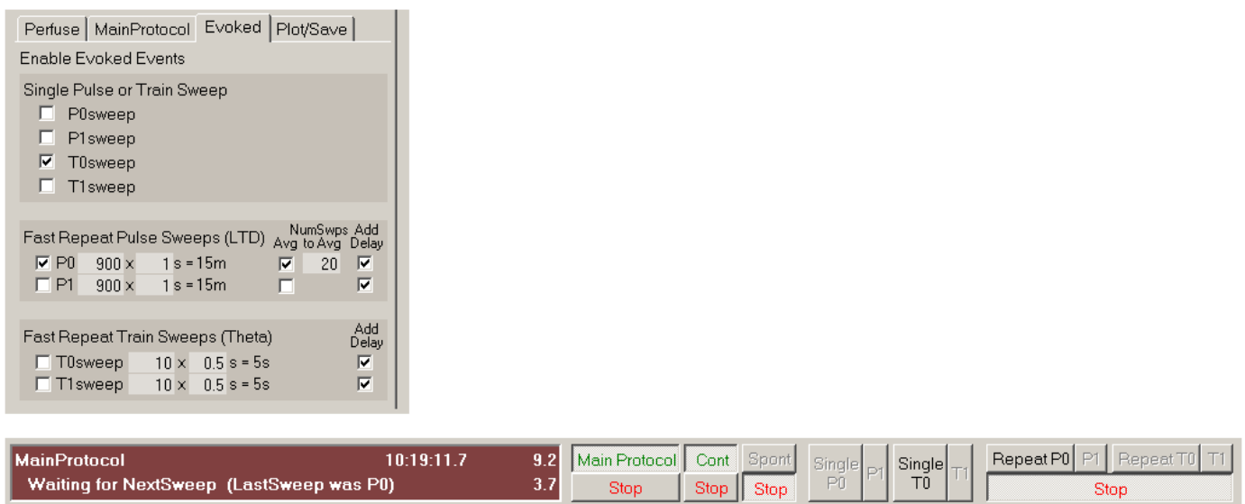
Fig. 4.4.2.1. EvokedEvents tabsheet showing which Single Sweeps and which Repeat Sweeps are enabled by checking the checkbox on the left. In this example, the Single T0sweep and Repeat P0sweeps are enabled and only the 'Single T0' and 'Repeat P0' Run Buttons at the bottom are enabled and ready to be clicked on.
