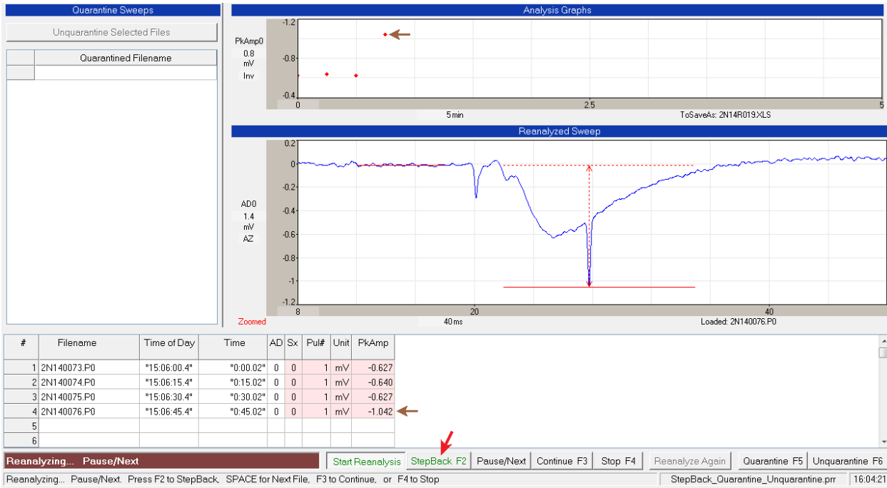
Fig. 14.7.2. Clicking on the 'StepBack F2' button (red arrow) or pressing the F2 key causes the analysis to StepBack one sweep to the sweep containing the artifact (2N140076.P0) that has a substantially larger peak amplitude (see the red amplitude detection line). The last data point in the analysis graph and the last line in the spreadsheet have been removed. The data point and spreadsheet line of the artifact sweep are marked by a brown arrow.
