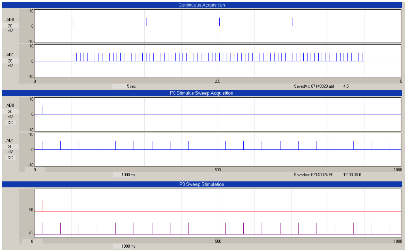
Fig. 13.3.1. An example of no time between sweeps. Note that there is no delay in the 20 Hz S1 stimulation between P0sweeps (AD1 trace in Continuous Acquisition panel).
