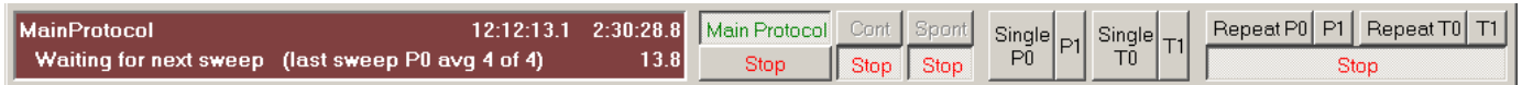
Fig. 3.1.5.1. Run Panel (left) and Run Buttons (right). The Run Buttons show full functionality for the Standard and Advanced Modes.
