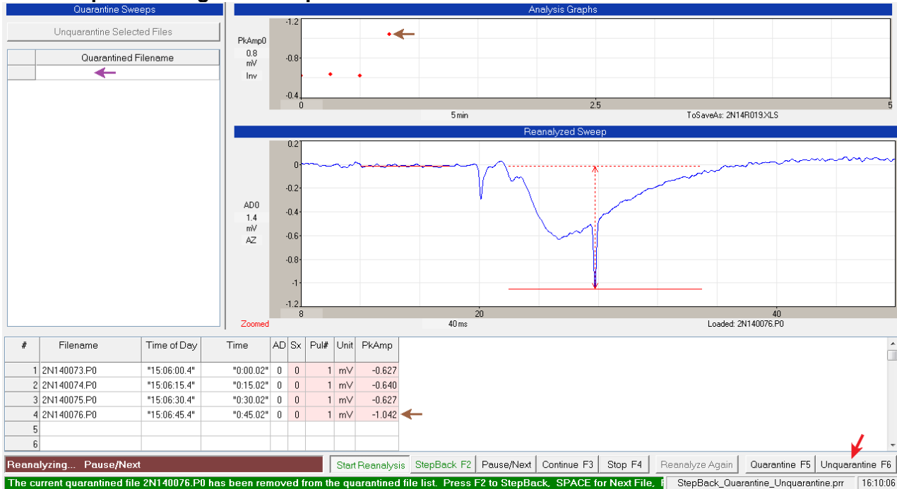
Fig. 14.14.3. Clicking the 'Unquarantine F6' button (red arrow) or pressing the F6 key unquarantines the current file (2N140076.P0), removes the filename from the Quarantined Filename spreadsheet (purple arrow), and reanalyzes the file and adding the 2N140076.P0 line to the spreadsheet and the data point to the analysis graph (brown arrows).
