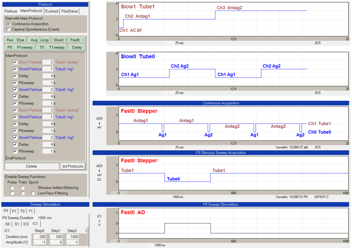
Fig. 10.4.1.4. Running the Dual-Line/Stepper example. The 'Slow0 Perfuse' and 'Slow1 Perfuse' events in the Protocol Builder (upper left) show when the Slow0/Tube0 and Slow1/Tube1 solutions are changed. The upper right panel shows the Slow1 Tube1 switch from 'Ch1 ACSF' to 'Ch2 Antag1' to 'Ch3 Antag2'. The next panel below shows the Slow0 Tube0 switch between 'Ch1 Ag1' and 'Ch2 Ag2'. The 'Continuous Acquisition' and the 'P0 Stimulus Sweep Acquisition' panel show recordings of the AO1 voltage shifts changing to Ch1 Tube1 or Ch0 Tube0. This results in the solutions switching between Antag1, Ag1 Antag1, Ag2, then Antag2 Ag1 Antag2 Ag2. The Sweep Stimulation bottom panels show change of AO1 (ie IC1) voltage output during a sweep. The -1V means to take whatever the current Fast0 output is BETWEEN sweeps (and when the MainProtocol is off), ie 1V or Ch1.
