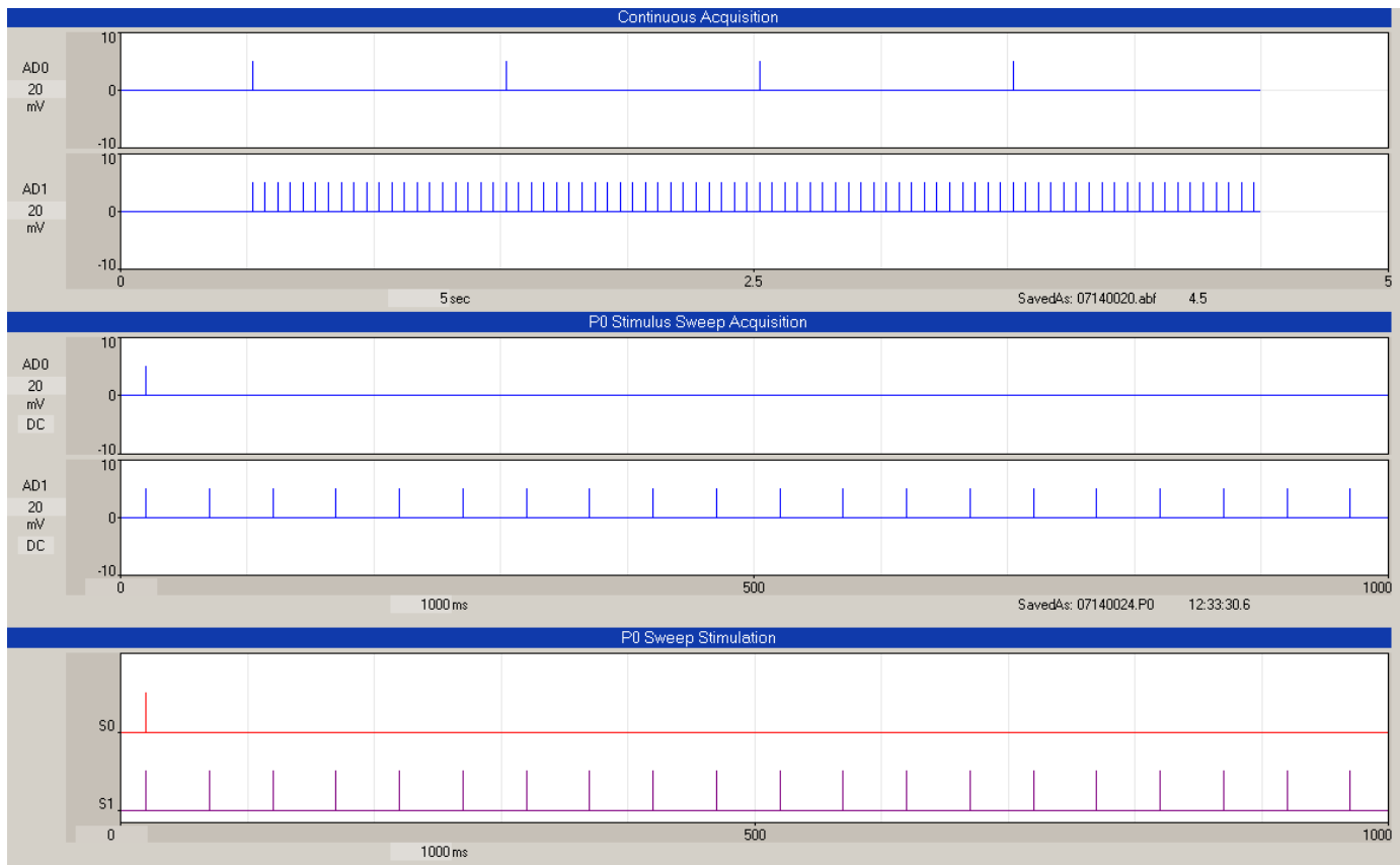
Fig. 13.5.1. An example of no time between sweeps. Note that there is no delay in the 20 Hz S1 stimulation between P0sweeps (AD1 trace in Continuous Acquisition panel).
