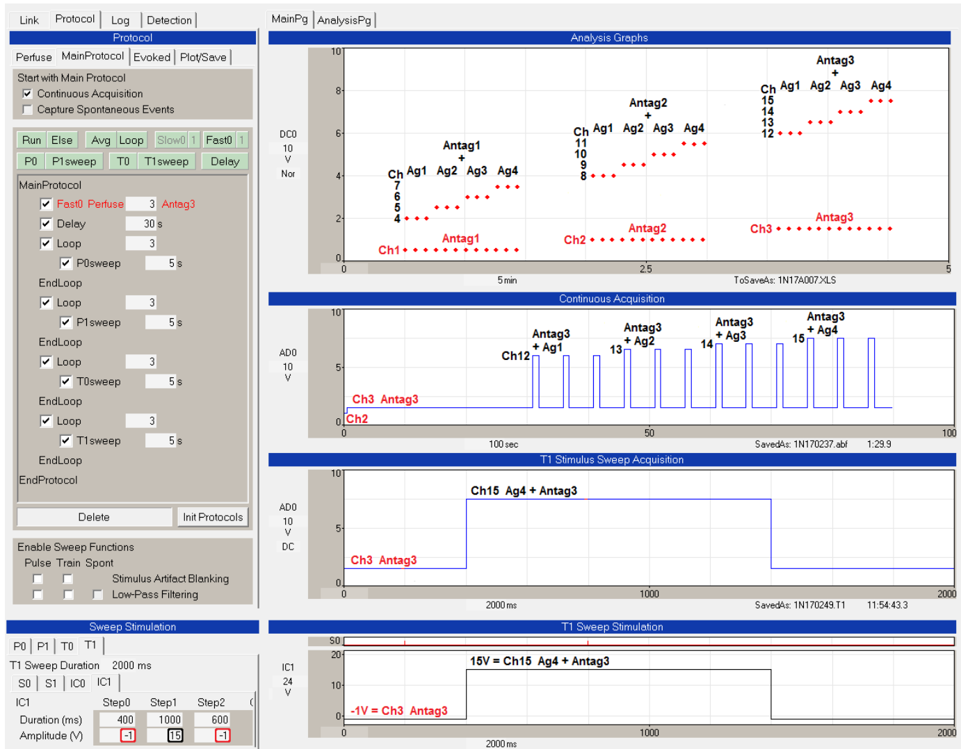
Fig. 9.3.2.1. An example of using Protocol Linking with Fast Perfusion to link 3 different protocol files to continuously perfuse solutions containing 3 different antagonist concentrations, and momentarily rapidly apply 4 different agonist concentrations with the different antagonist concentrations - ie apply 15 different solutions. Uses 16ch AO1 with a Gain of 0.5. See FastPerfusion1.pro , FastPerfusion2.pro , and FastPerfusion3.pro . To use connect AnalogOut1 (AO1) to AnalogIn0 (AI0 or AD0).
