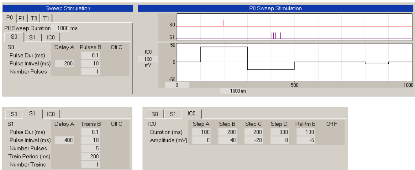
Fig. 4.7.2.4. Extracellular heterosynaptic primed burst stimulation (S0 single pulse, S1 train) and coincident intracellular (IC) depolarization and hyperpolarization stimulation with an RsRm test pulse.
