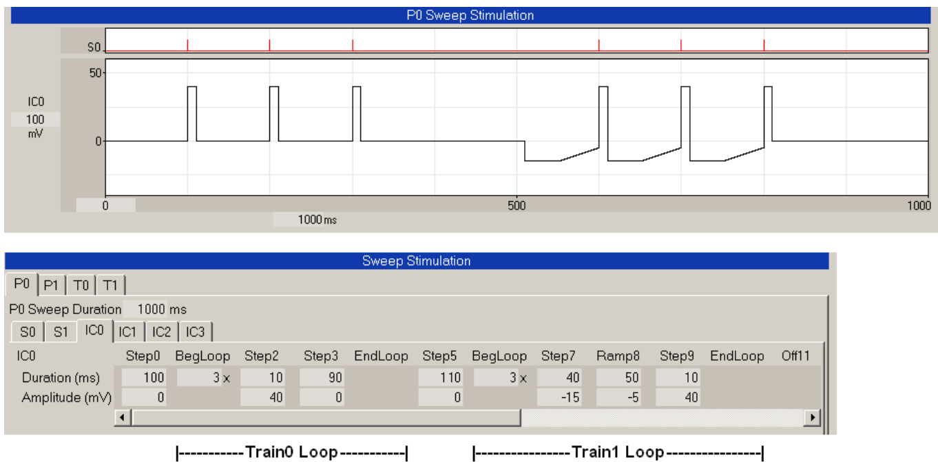
Fig. 4.9.2.5. Sequential Single Trains using BegLoop/EndLoop constructs for Train0 Loop and Train1 Loop. Also note that ramps are generated within the Train1 Loop.
