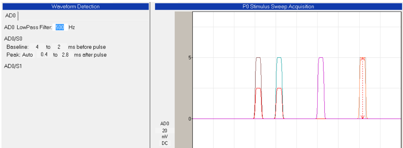
Fig. 5.6.1. Changing the low pass filtering value for channel AD0 in the Waveform Detection panel from 200 Hz (Figs. 5.1.1 through to 5.5.2) to 500 Hz here changed the filtering of all the Viewed (magenta trace), the single Imposed (brown, cyan and orange traces) and the Averaged/Imposed (red trace) Sweeps, as well as the underlying Current Acquired Sweep's low-pass filtered trace (underlying the orange trace). The sweep duration is 100 msec. Compare this with the 200 Hz low-pass filtered traces in Fig. 5.5.1.
