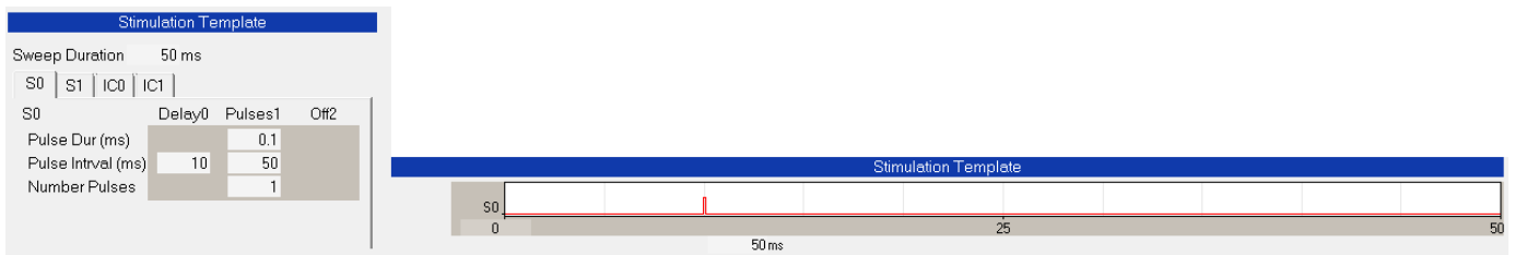
Fig. 14.5.2. The Stimulation Template consisting of Screen Fields on the left, and stimulation graphs on the right (only S0 graph is used and shown). The key field is the 'Delay A' Pulse Interval (pulse delay) field.
